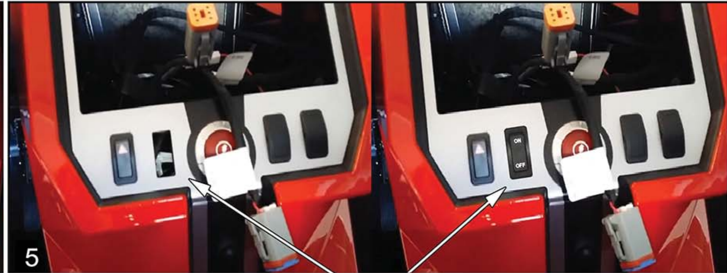
5 Remove the switch knockout plate in your dash and insert the new ON / OFF factory style rocker switch included in the kit.
