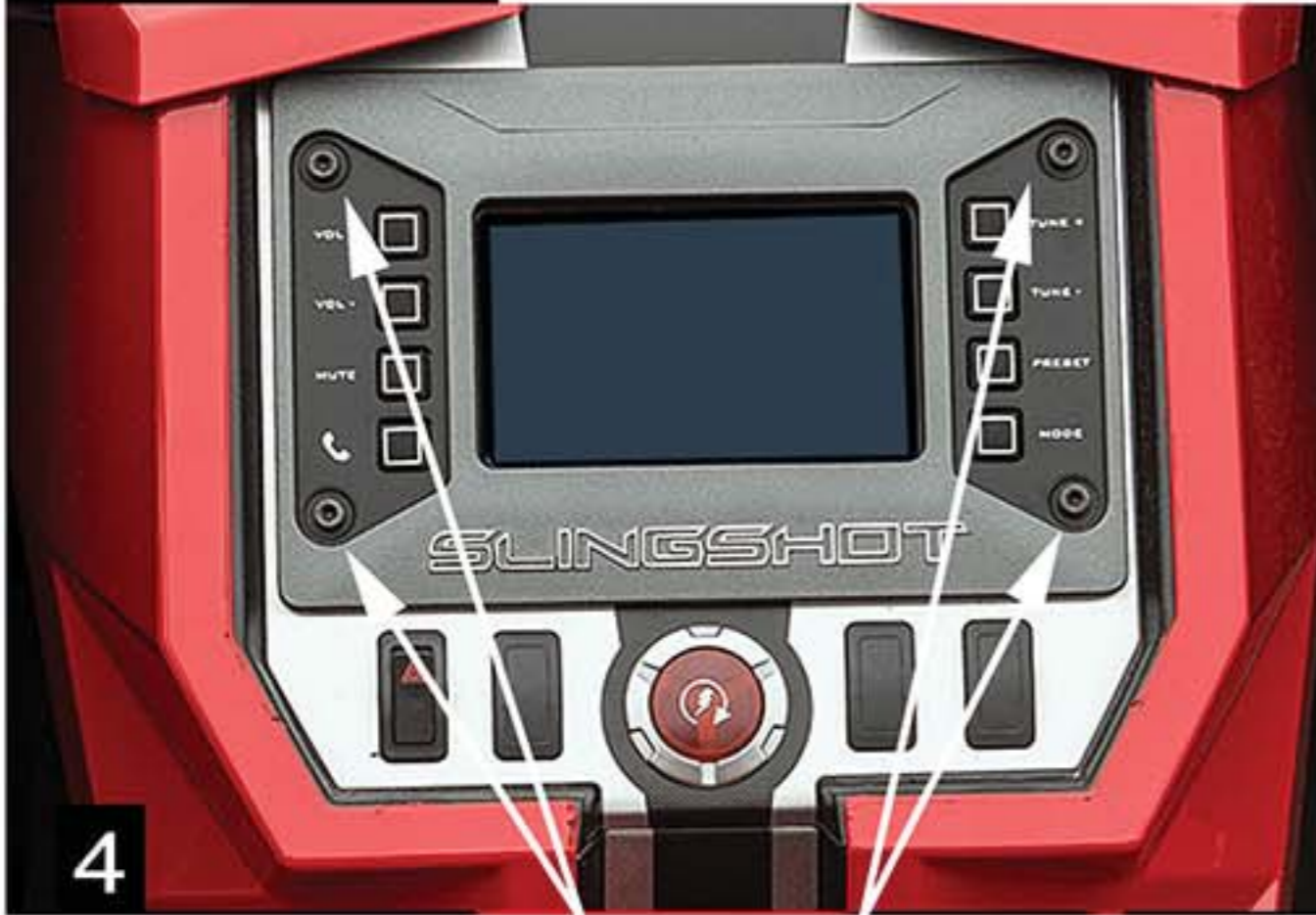
4 Remove 4 face plate bolts and unplug and remove the Slingshot Infotainment Center
